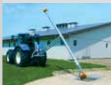
Slurry Mixer for covered slurry pits
