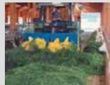
Green Fodder Distributor for feeding passage in the stable
